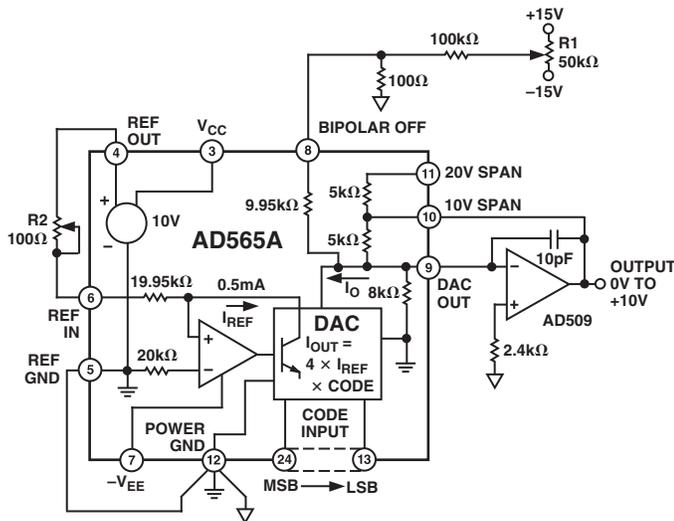
Figure 1. 0 V to 10 V Unipolar Voltage Output
