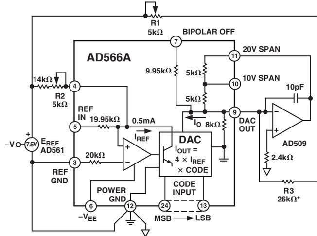
\* THE PARALLEL COMBINATION OF THE BIPOLAR OFFSET RESISTOR AND R3 ESTABLISHES A CURRENT TO BALANCE THE MSB CURRENT. THE EFFECT OF TEMPERATURE COEFFICIENT MISMATCH BETWEEN THE BIPOLAR RESISTOR COMBINATION AND DAC RESISTORS IS EXPANDED ON PREVIOUS PAGE.
