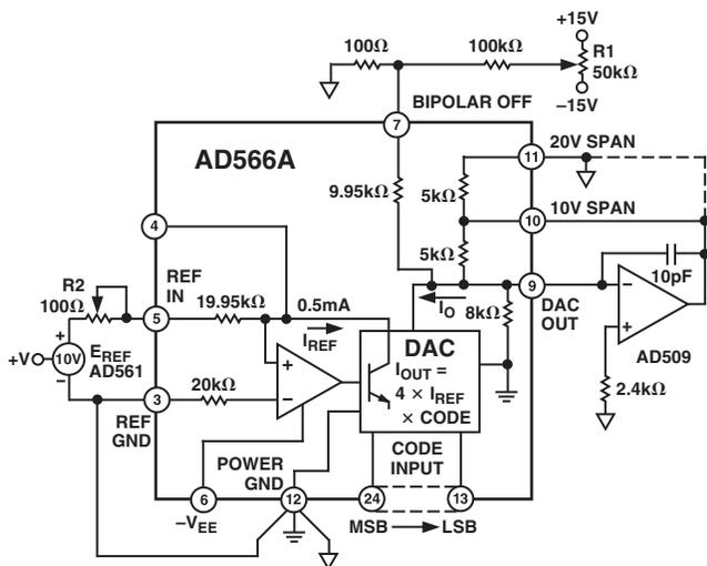
Figure 4. 0 V to 10 V Unipolar Voltage Output
