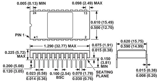
CONTROLLING DIMENSIONS ARE IN INCHES; MILLIMETER DIMENSIONS (IN PARENTHESES) ARE ROUNDED-OFF INCH EQUIVALENTS FOR REFERENCE ONLY AND ARE NOT APPROPRIATE FOR USE IN DESIGN
