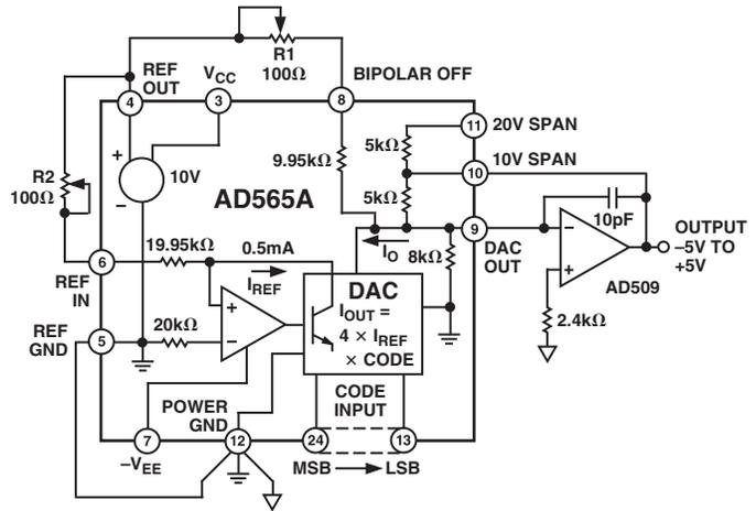
Figure 2.  $\pm 5$  V Bipolar Voltage Output
