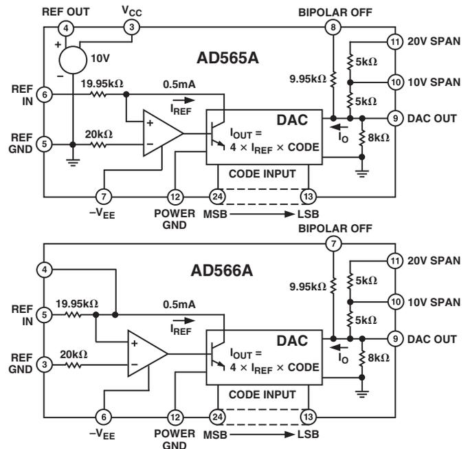
AD565A and AD566A are available in four performance grades. The J and K grades are specified for use over the  $0^\circ\text{C}$  to  $+70^\circ\text{C}$  temperature range while the S and T grades are specified for the  $-55^\circ\text{C}$  to  $+125^\circ\text{C}$  range. The D grades are all packaged in a 24-lead, hermetically sealed, ceramic, dual-in-line package. The JR grade is packaged in a 28-lead plastic SOIC.
