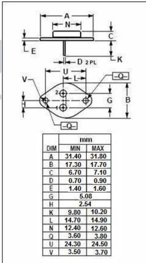
**isc Silicon NPN Power Transistor****AD161****ELECTRICAL CHARACTERISTICS**T<sub>j</sub>=25°C unless otherwise specified
