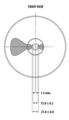
Plastic Reel Format (all dimensions are in millimeters)
