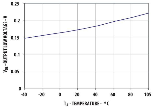
Figure 5. V<sub>OL</sub> vs. temperature
