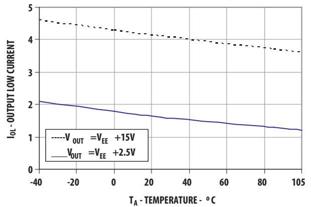
Figure 3. I<sub>OL</sub> vs. temperature
