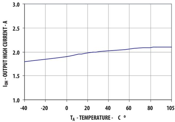
Figure 2. I<sub>OH</sub> vs. temperature
