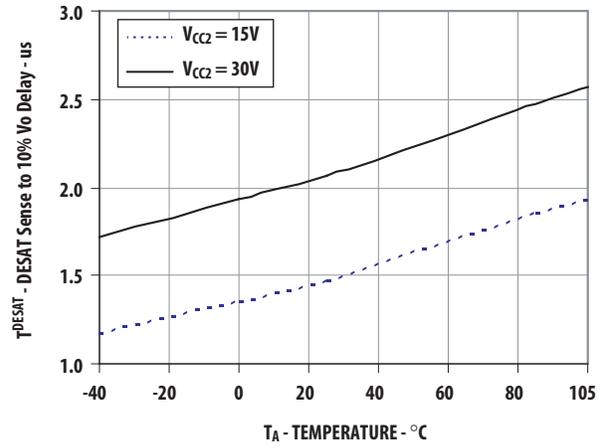
Figure 18. DESAT sense to 10% VOUT delay vs. temperature
