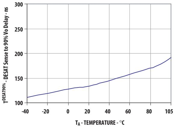
Figure 17. DESAT sense to 90% VOUT delay vs. temperature
