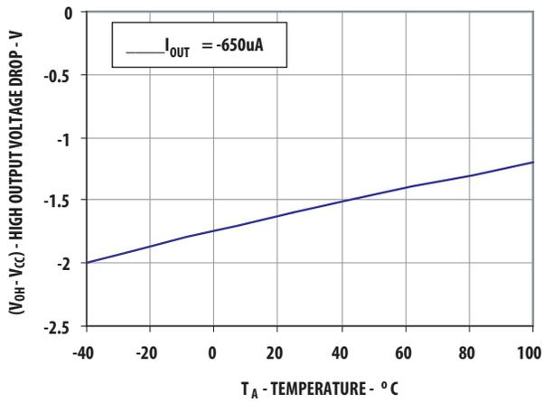
Figure 4. V<sub>OH</sub> vs. temperature
