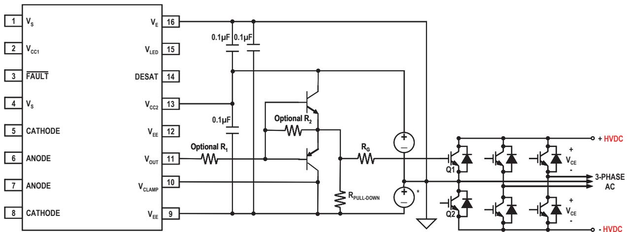
**Figure 40.** IGBT drive with negative gate drive, external booster and desaturation detection ( $V_{CLAMP}$  should be connected to  $V_{EE}$  when it is not used)  $V_{CLAMP}$  is used as secondary gate discharge path. \* indicates component required for negative gate drive topology
