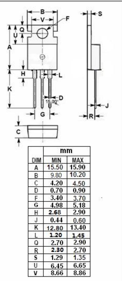
**isc Three Terminal Negative Voltage Regulator****7905****• ELECTRICAL CHARACTERISTICS** $T_j=25^\circ\text{C}$  ( $V_i = -10\text{V}$ ,  $I_o = 0.5\text{A}$ ,  $C_i = 2.2 \mu\text{F}$ ,  $C_o = 1 \mu\text{F}$  unless otherwise specified)
