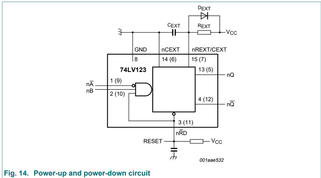
Fig. 14. Power-up and power-down circuit
