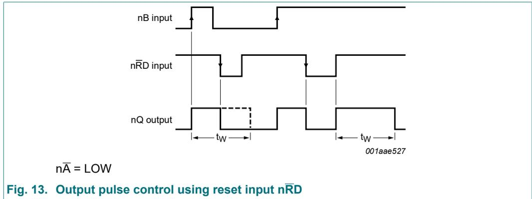
Fig. 13. Output pulse control using reset input  $n\bar{RD}$
