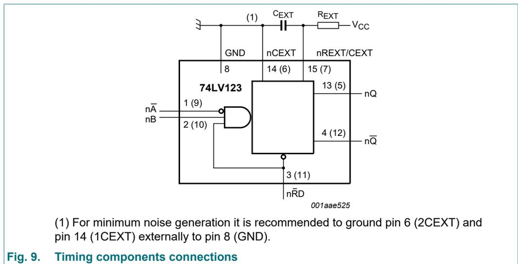
Fig. 9. Timing components connections
