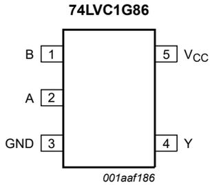
Fig. 4. Pin configuration SOT353-1 (TSSOP5) and SOT753 (SC-74A)
