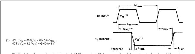
Fig.6 Waveforms showing the clock (CP) to output (Q<sub>n</sub>) propagation delays, the clock pulse width, output transition times and the maximum clock pulse frequency.
