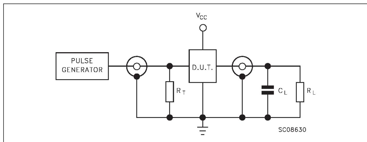
C<sub>L</sub> = 50 pF or equivalent (includes jig and probe capacitance)
