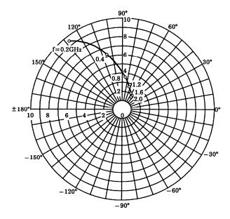
$S_{12e}$   $V_{CE} = 10V$   $I_{C} = 5mA$   $Ta = 25^{\circ}C$
