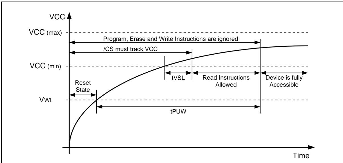
Figure 57. Power-up Timing and Voltage Levels
