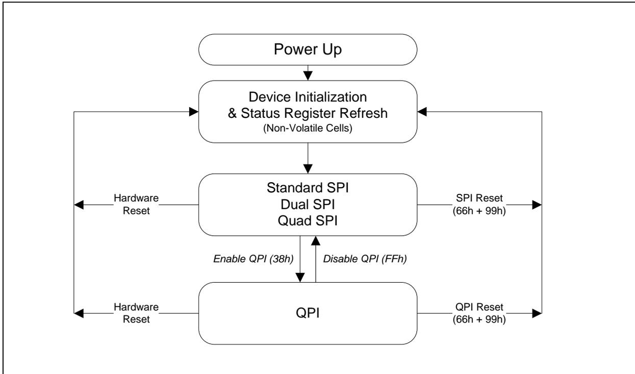
Figure 3. W25Q128FW Serial Flash Memory Operation Diagram
