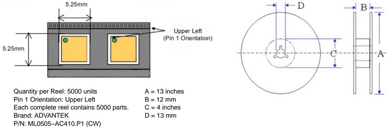
**Figure 13. Package Orientation on Tape**
