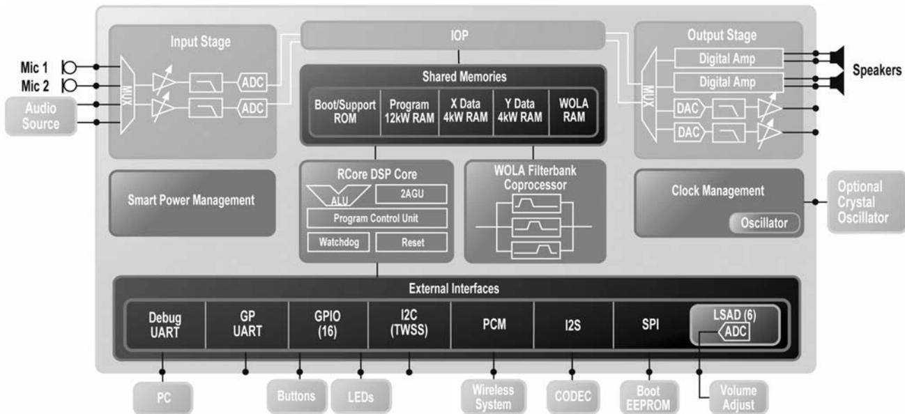
Figure 2. BELASIGNA 250 Architecture: A Complete Audio Processing System
