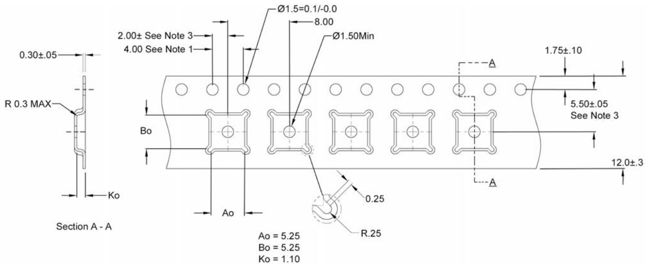
1. 10 sprockets hole pitch cumulative tolerance  $\pm 0.2$ .
